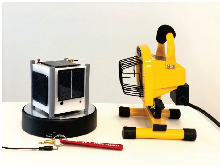
Turntable and Lamp used to Simulate On Orbit Rotation
